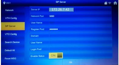
Sip server to be set to VTO's IP address, leave all settings as default, only Enable status to "ON"
