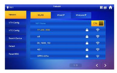
Select WLAN, Swipe OFF, to switch ON WLAN, Select the Wireless you want to connect to and insert password
