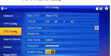
For VTO Setup, Insert IP / user name and password of VTO , then switch Enable status to ON. You can also search for devices to add on the next tab.
