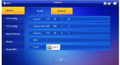
Set Network settings / or Enable DHCP, recommended to set as STATIC, "DHCP=OFF".
